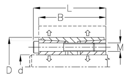
$\begin{array}{lll} \text{B mm} & = 202 \\ \text{d H8 mm} & = 360 \\ \text{D mm} & = 455 \\ \text{Fit tolerance} & = \text{Aksel h8, Nav H8} \end{array}$
